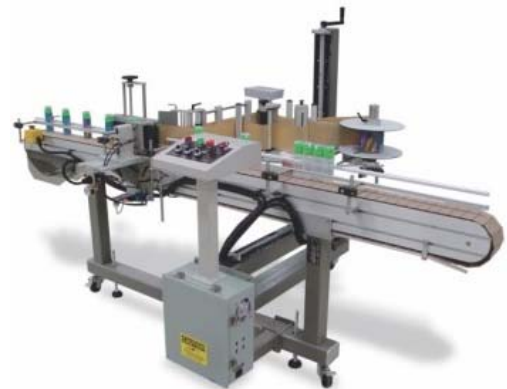
Open frame labeling system outfitted with a three-roller capture device for orientation labeling
