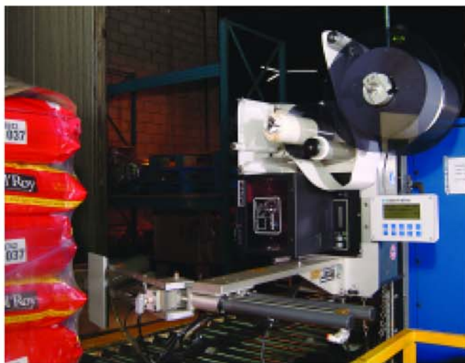
The Label-Aire printer/applicator was customized to properly affix labels on the pallets shipped from the Nestlé Purina plant.
